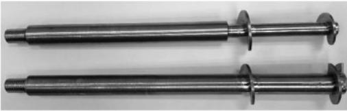
Figure 2. Photograph of optimised (upper) and standard uniform (lower) screw piles tested in the centrifuge.
