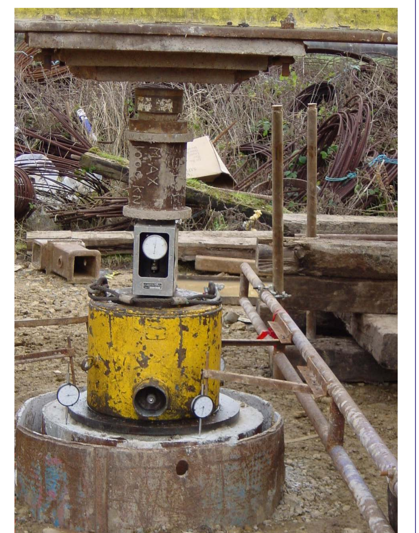
Figure 9. Example of field testing of pile capacity.
