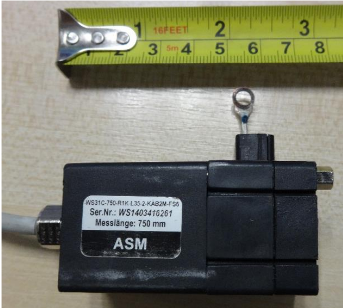
Figure 3. Draw-wire potentiometer WS31C.
