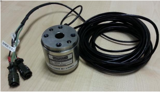
Figure 2. Novatech F310-Z axial force and torque transducer.
